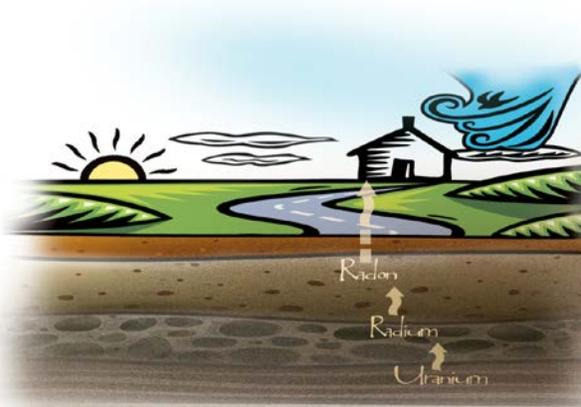
*Radon is a colorless, odorless, naturally occurring radioactive soil gas that can get into homes through foundations and cause cancer. 2 of 5 homes in Minnesota have high levels. Systems can be installed to reduce the amount of radon in buildings. [Read more.](#)*
